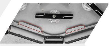
Our exclusive Aero Deck™ is .270-inch fabricated steel & features fully adjustable baffles enabling you to customize your cut to various grass conditions. Available in 54″, 61″, 66″ & 72″ widths.
