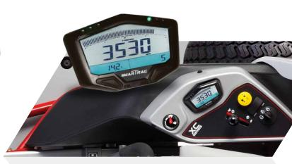
SmarTrac™ Monitoring System features a tachometer and resettable hour meter, with alerts for low oil pressure and overheating.
